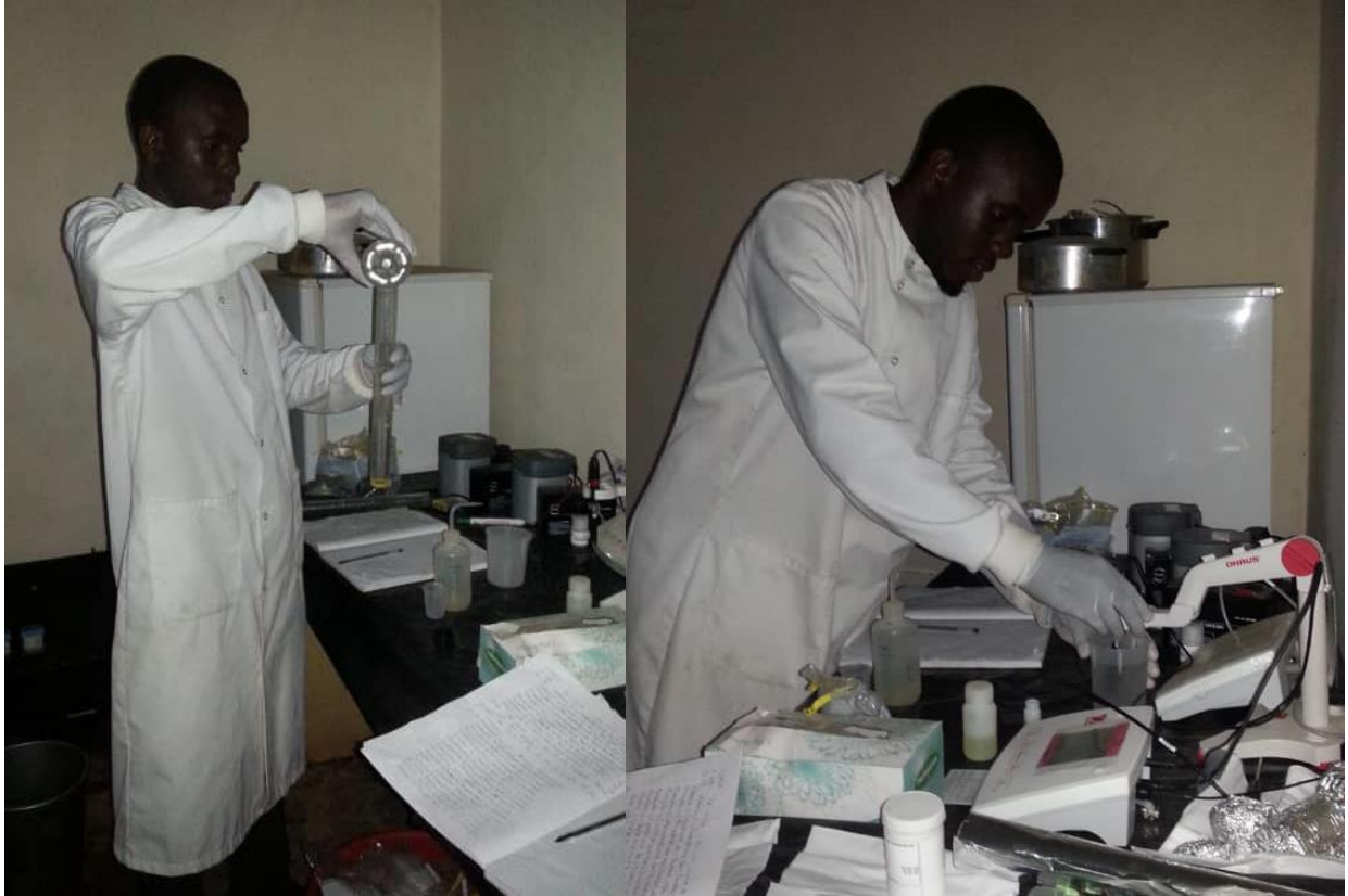
Figure 3: Analysis of turbidity (left), TDS, EC and salinity (right) in the field laboratory
